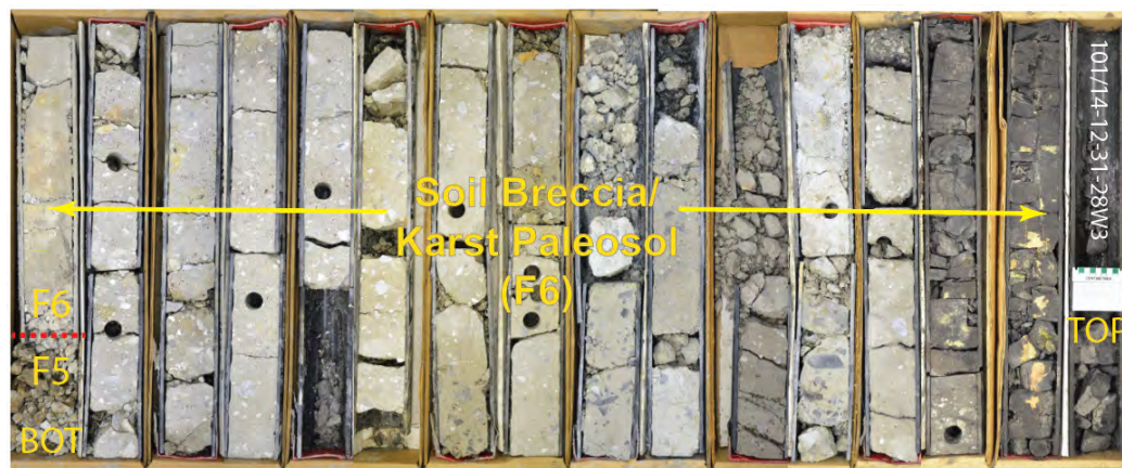
Figure 5 – Core 4 from well 101/14-12-031-28W3; 85K078 illustrates the contact between facies 5 (F5) and 6 (F6). Core 4 shows the soil breccia/karst paleosol facies association (FA4) and the stacking relationship with facies 5 (epikarst facies association (FA3)). Notably, the chert clasts within FA4 change from white to dark grey and black towards the top of the unit. Facies association 4 is commonly capped with a coal.
